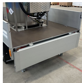
Platform made of marine plywood
